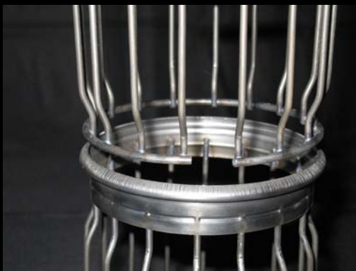
Split Ring - Slide the latch up the top piece (away from the connecting end), then squeeze the end ring until it rests in the mating groove on the bottom section ring. Slide the latch down.
