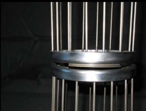
Royal Twist-Lok™ - When joining round cages, hold the ends in position and hand-tighten in a clockwise direction. Simply twist counter-clockwise to separate the sections.
