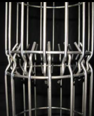
Finger Style – Traditional method for joining multi-section cages. Align the top section atop the bottom, and snap the two together with firm hand pressure or locking pliers.
