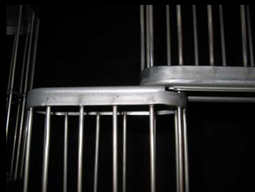
Royal Slip-Lok™ - Position the joining ends of oval cages together, slightly offset, so the flat collar surfaces are together, and slide into position.
